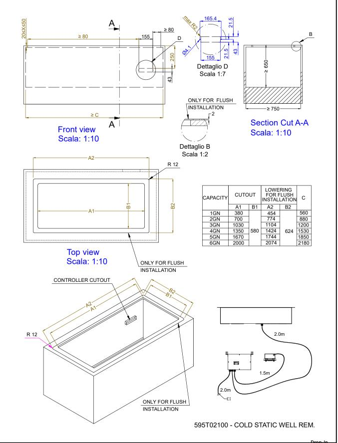
Drop-in remote refrigerated well, static (4 GN container capacity)
