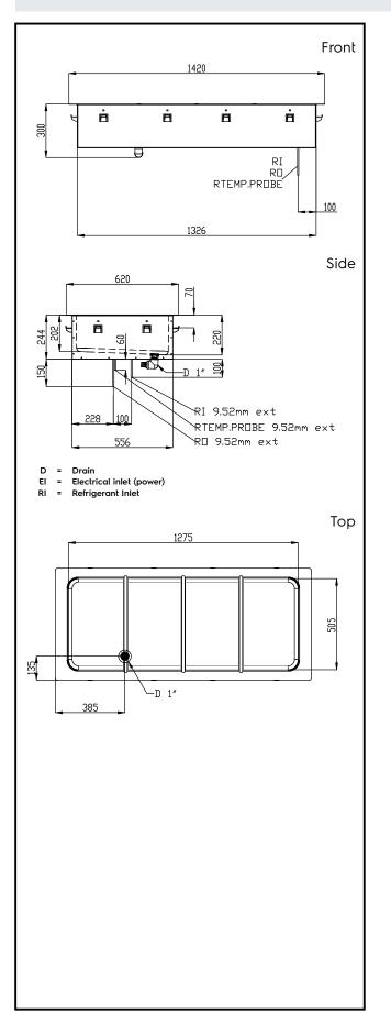
Drop-In Drop-in remote refrigerated well, static (4 GN container capacity)
